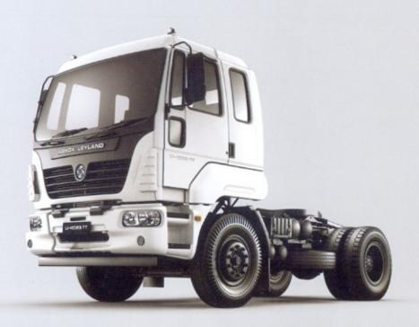
THE U-4023 TT IS DESIGNED TO TRANSPORT A WIDE VARIETY OF GOODS. POWERED BY AN EFFICIENT 'H' SERIES COMMON RAIL FUEL INJECTION SYSTEM (CRS) ENGINE AND SUPPORTED BY A MATCHING DRIVELINE, THE U-4023 TT ENHANCES PRODUCTIVITY AND OFFERS FASTER TRIP TIME. ALSO, ITS FULLY-SUSPENDED SLEEPER CAB REDEFINES THE LONG-HAUL EXPERIENCE. THESE FEATURES ARE WHAT MAKE THE U-4023 TT THE BEST 40-TONNER IN ITS CLASS.
